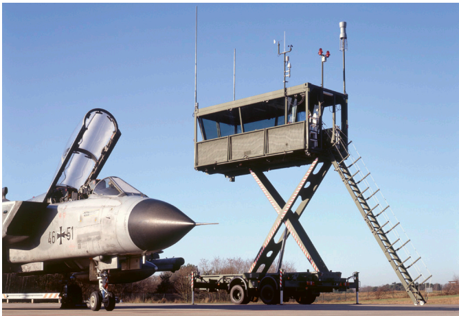
R&S®M3SR Series4400 in a mobile ATC tower
